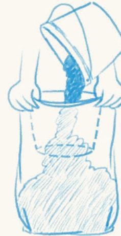
Before filling, the bottom of the feed bag was positioned exactly where it was needed on the wall. Once all 4 buckets were in the bag, the top of the bag was folded over 3-4 times creating a 2" flap that was stapled shut. The bag was then lowered squarely into position on the wall.
