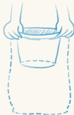
*earth is poured through the bucket into the bag*
